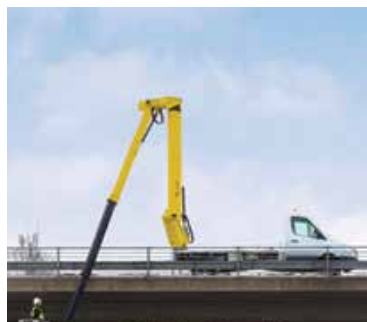
The ability to work over rooftops to access difficult to reach areas is aided by a flat bottomed basket
